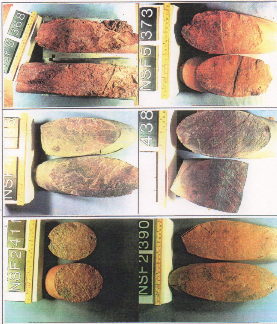
Figure 3.8 Photographs of joints in BVG, BH2, BH4 and BH5, from depths between 570 m and 796 m. Examples of steepest (J1) joints (top left), four J2 joints (dip 50-75°) and one J3 joint (bottom left) (NGI 901038-18/2 and 28/7, NGI 931005-11/1)
